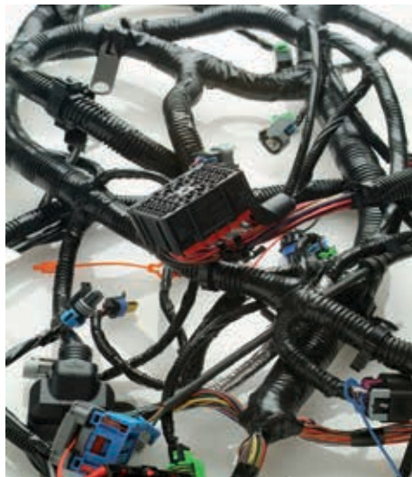
Figure 89: Automotive cable harness – source: Lear
