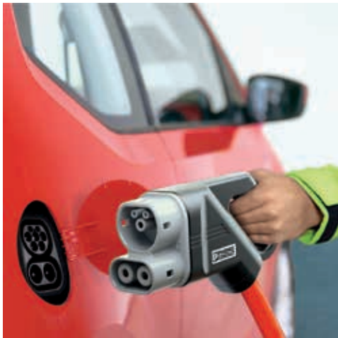
Figure 93: AC/DC charging plug with Combined Charging System (CCS) – source: Phoenix Contact
