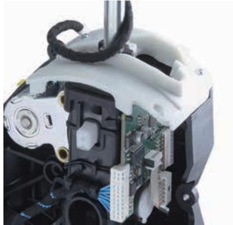
Figure 88: RAST connectors in the gear selector of an automatic drive – source: Lumberg
