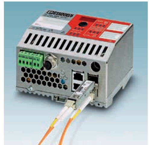
Figure 56: Field device with data interfaces (fibre-optic and copper) – source: Phoenix Contact
