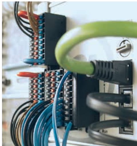
Figure 55: I/O element (input/output) with sensor connectors – source: Weidmüller
