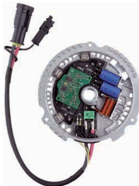
Figure 43: Connectors and contact elements in a cooling fan control unit for a car – source: Lumberg
