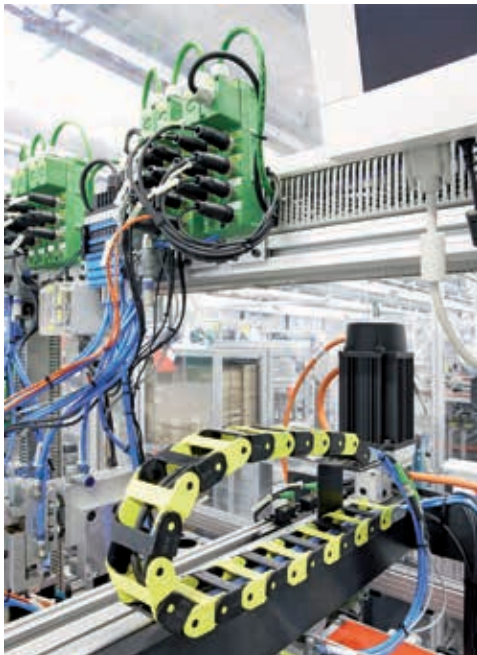
Figure 51: Sensor/actuator distributor in production automation – source: Phoenix Contact
