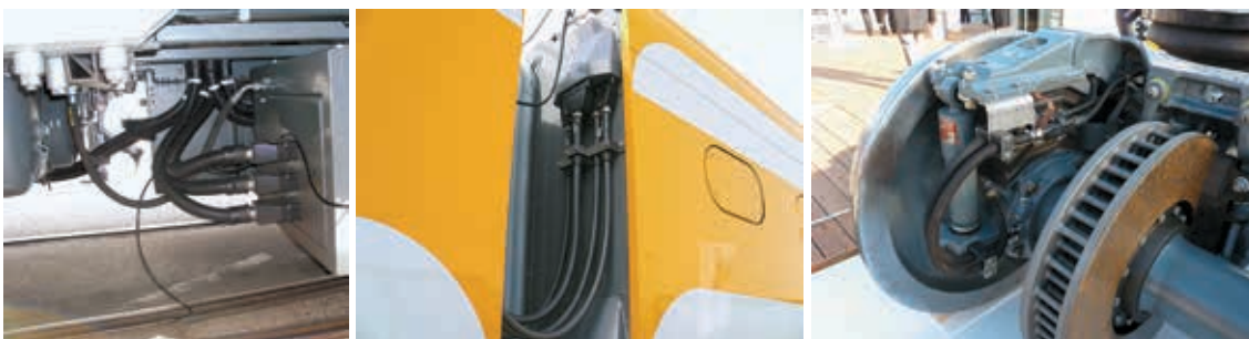
Figure 64 to 66: Robust connectors for the railway industry – undercarriage container (left), carriage transition (centre) and temperature sensor for the brakes (right) – source: Harting
