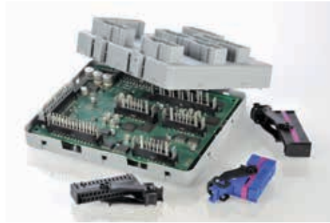
Figure 87: On-board electronics control units with connectors – source: Lear
