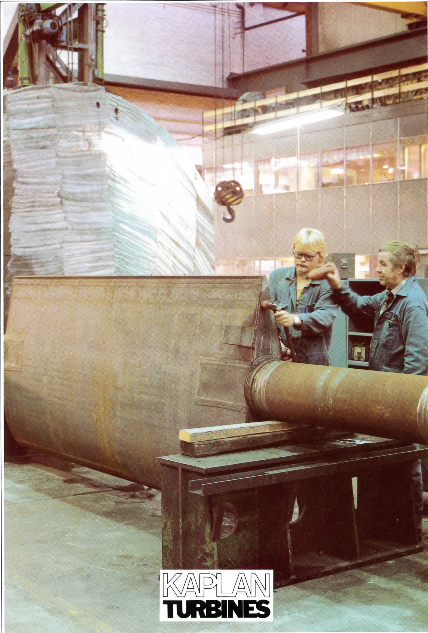
Guide vane and runner blade for 8.3 m runner diameter Kaplan turbine
